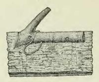
In some fishing craft the planks are tied to the frames by ropes through holes in the under side of the frames and corresponding holes or in cleats projecting from the planks.
